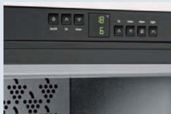
The wine cabinets are equipped with an accurate **electronic control system** with digital temperature display. These appliances incorporate a special climate control system that can layer the temperatures. In the upper zone, for example, red wine can be kept at +16°C to +18°C while the lower zone is set at an ambient temperature of +5°C to +7°C.
